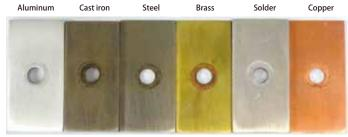
Case of coolant which has low anti-corrosion quality
