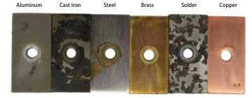
There are lots of corrosion on manu of the test pieces which can cause overheating due to corrosion clogging, leakage etc of the radiator.
