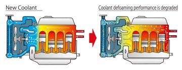
Degraded coolant loses antifoaming performance and foam will obstruct coolant circulation in the cooling system. The radiator will not cool the engine effective and will cause overheating. In addition, it will increase the risk of radiator damage due to cavitation.
