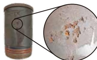
It is a corroded cylinder liner by cavitation which is caused by degraded coolant.
