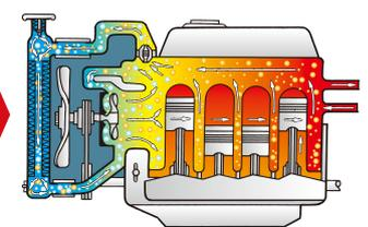
Degraded coolant loses antifoaming performance and foam will obstruct coolant circulation in the cooling system. The radiator will not cool the engine effectively and will cause overheating. In addition, it will increase the risk of radiator damage due to cavitation.
